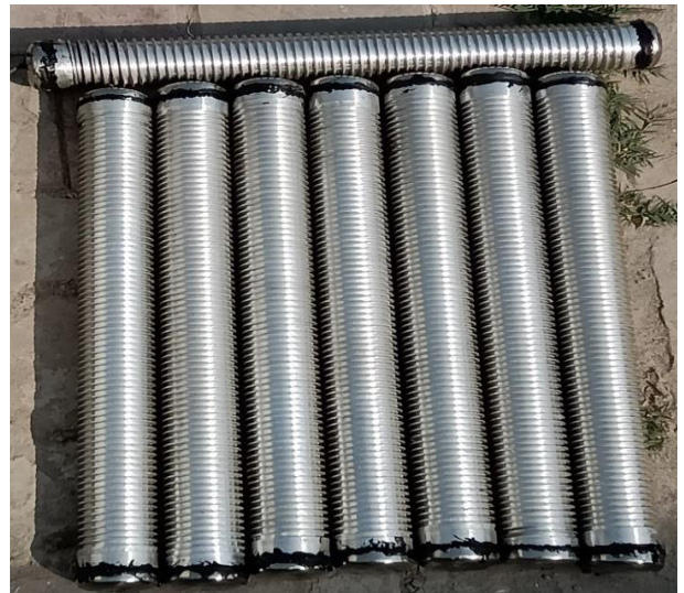
Figure 7. Aluminium Circular finned thermal storage pipe
