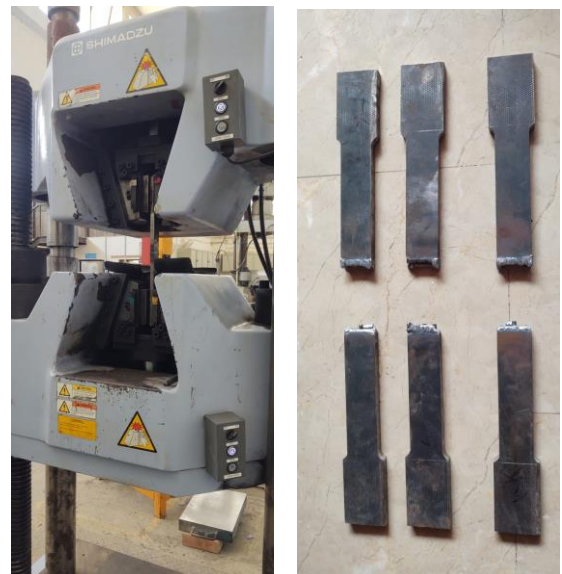
Figure 3. Tensile Test and Fractured Samples
