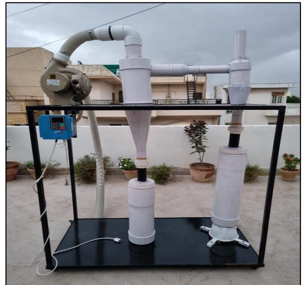
Figure 5. View of Particle Grading equipment with VFD and Blower on Left
