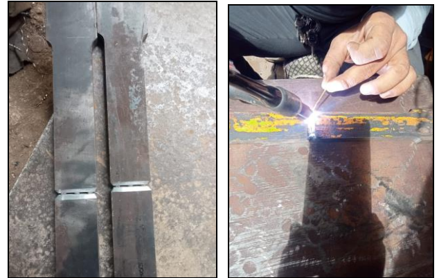
Figure 2. Argon Gas Welding on samples
