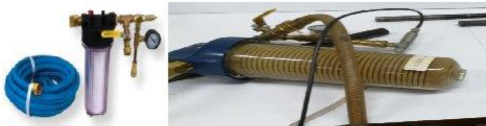
Figure 3. Water filter along with rpm controlling valve, pressure gauge and black wire to send and receive signals
