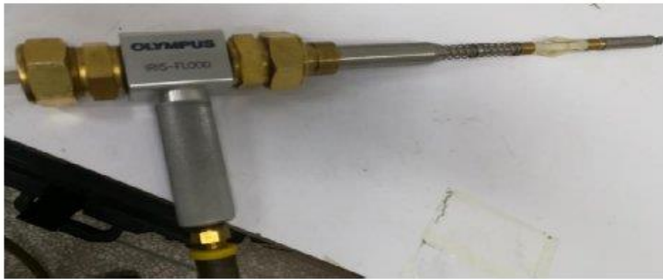
Figure 4. Complete arrangement of inspection probe, includes guide tube, plastic centering device, transducer and turbine turbine
