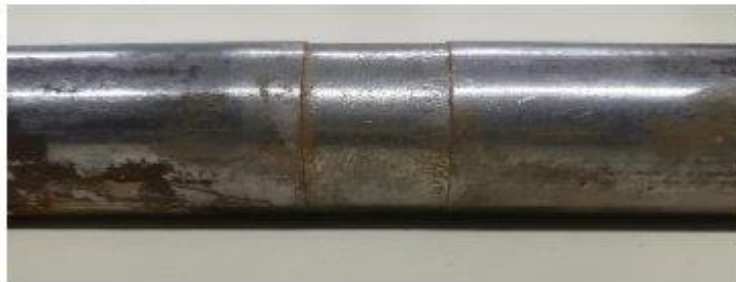
Figure 11. Actual Condition of defect 4 over the surface of tube.
