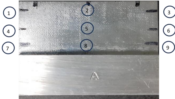
Figure 3. Sample Machined Thin Walls
