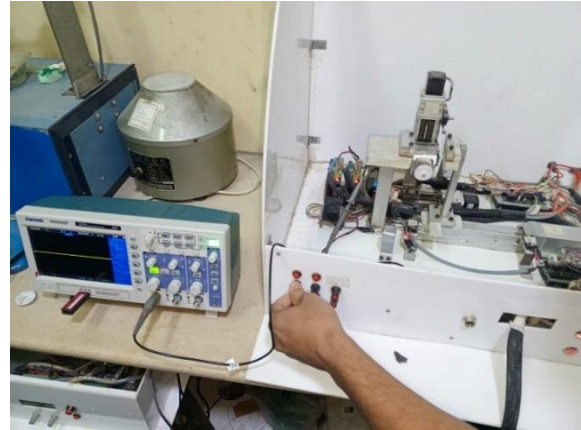
Figure 21. Thin film vibration testing machine CAM based
