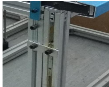
Figure 3. Slider Attached to the Leg of Adjustable Table
