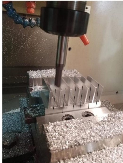
Figure 2. Machining of thin walls
