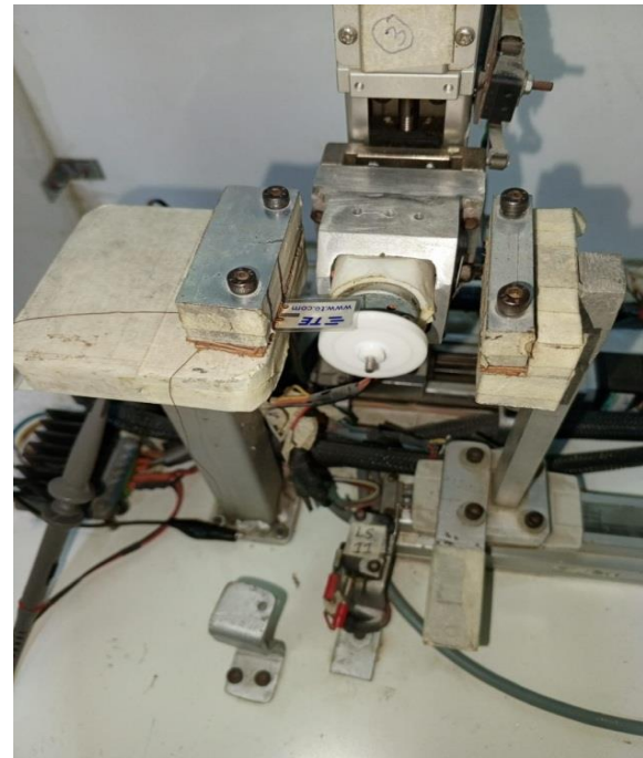
Figure 22. Single Device Mounted on thin film vibration testing machine
