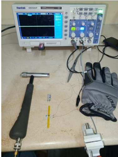
Figure 5. Impact Testing Setup
