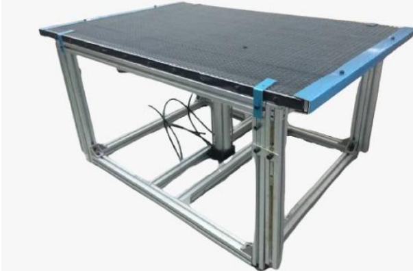
Figure 7. The Actual Fabricated Adjustable Table with the Honeycomb Panel and Double Acting Cylinder
