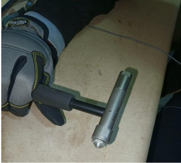
Figure 17. Impact Hammer with Aluminum Tip
