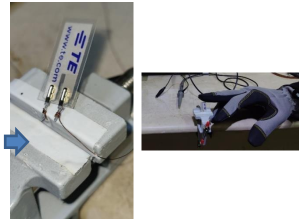
Figure 7. Flexing device up to 5-10 mm displacement with anti-static gloves
