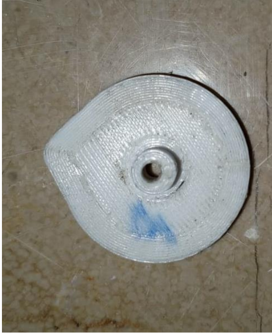
Figure 23. 3D printed, 3 mm Displacement CAM
