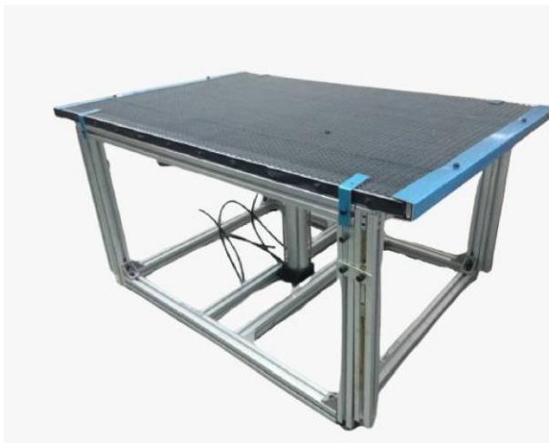
Figure 7. The Actual Fabricated Adjustable Table with the Honeycomb Panel and Double Acting Cylinder
