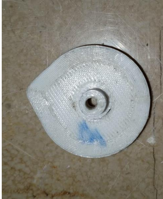
Figure 23. 3D printed, 3 mm Displacement CAM
